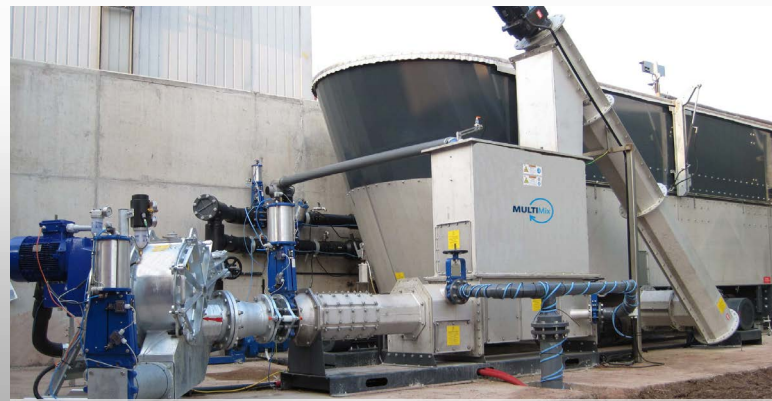
The MULTIMix comminutes substrates and separates extraneous materials.
