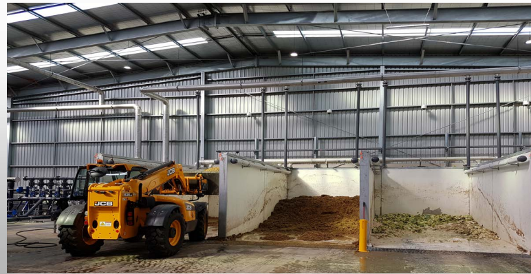
The digesters are continuously supplied with substrates from five prestorage tanks.
