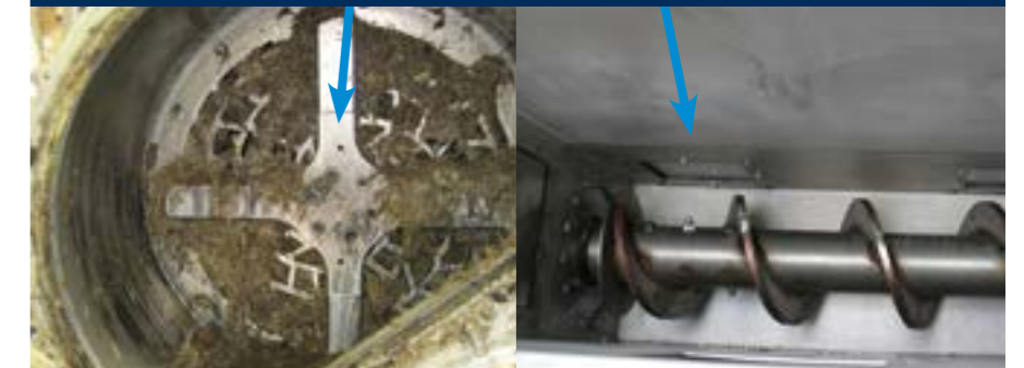
Bottom left: The macerator crushes sticky and lumpy materials effectively.
