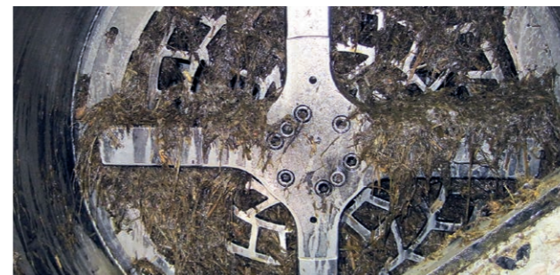
Macerator ensures reliable substrate shredding and separates extraneous materials.
