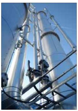
The plant in Ebsdorfergrund produces 1,000 standard  $m^3/h$  of raw biogas and efficiently conditions it to 550 standard  $m^3/h$  of natural gas equivalent biomethane.
